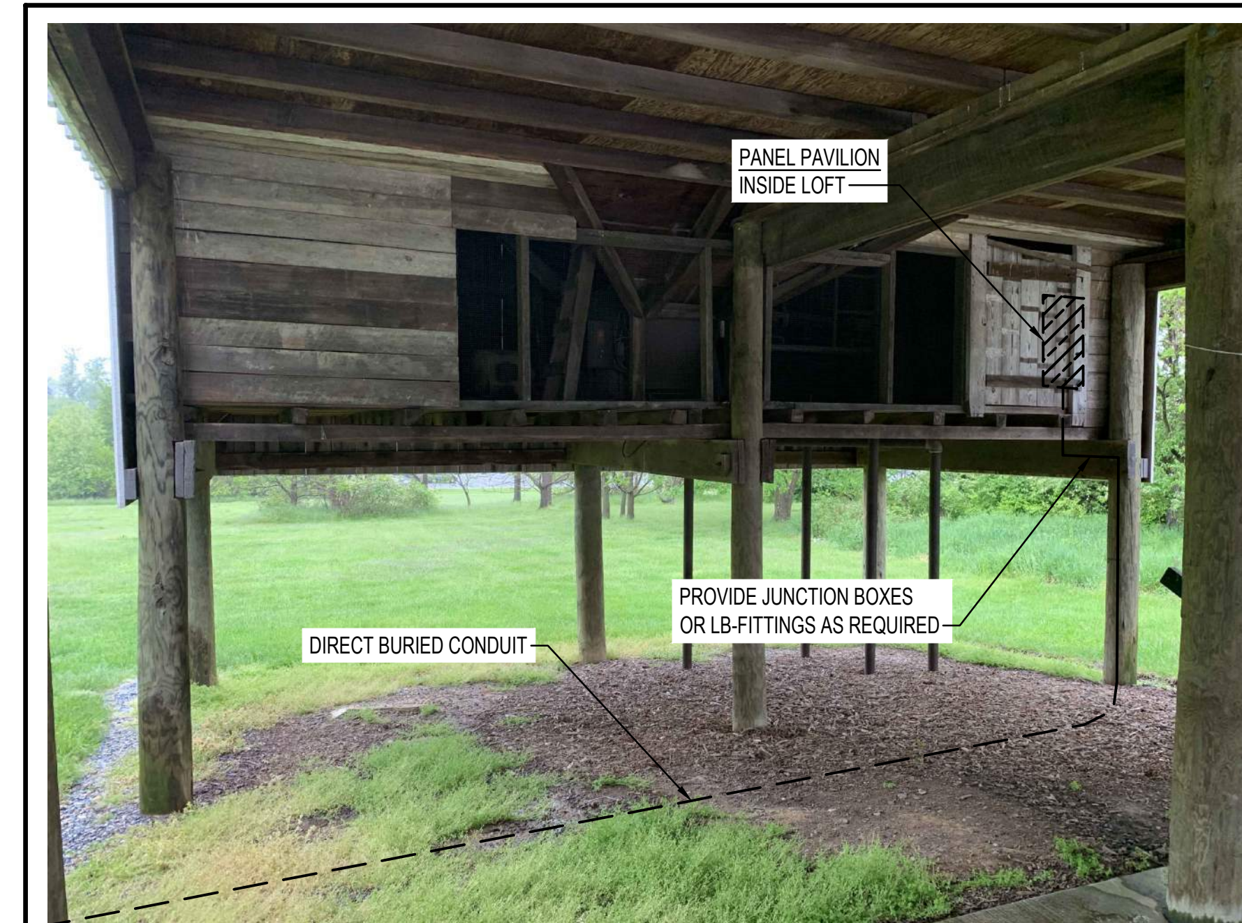
3 PAVILION PANEL INSTALLATION DETAIL E503 / NTS
