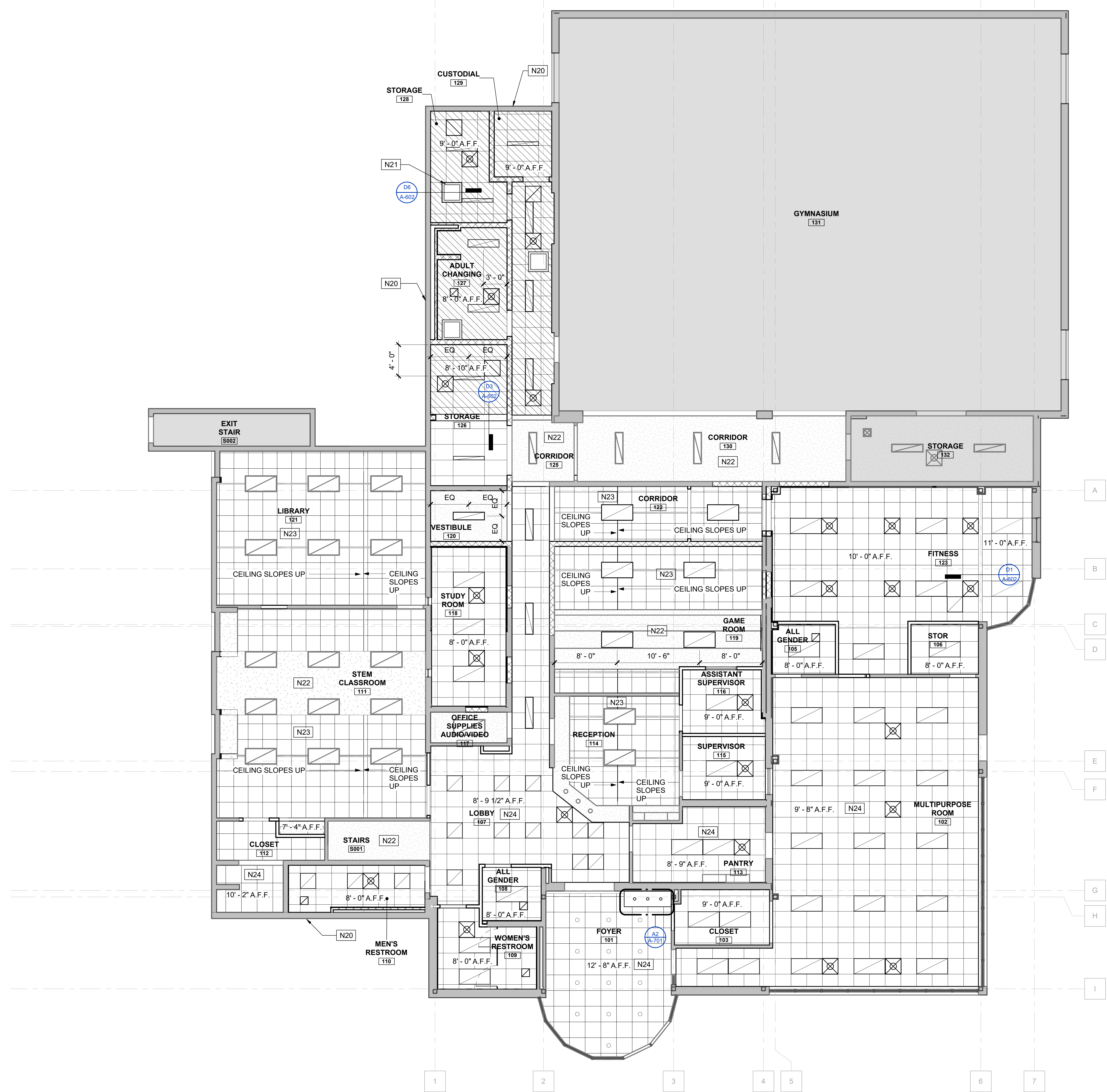
A1 FIRST FLOOR RCP - NEW WORK A-151 3/16" = 1'-0"
