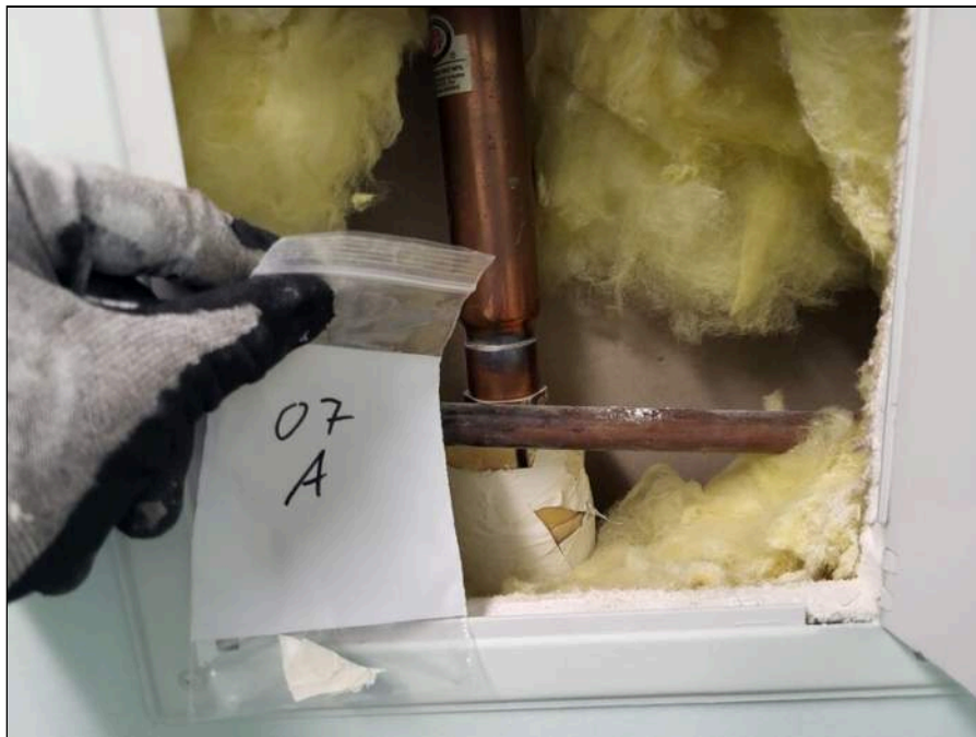
38 - Endcap Mastic on Paper over Foil TSI
