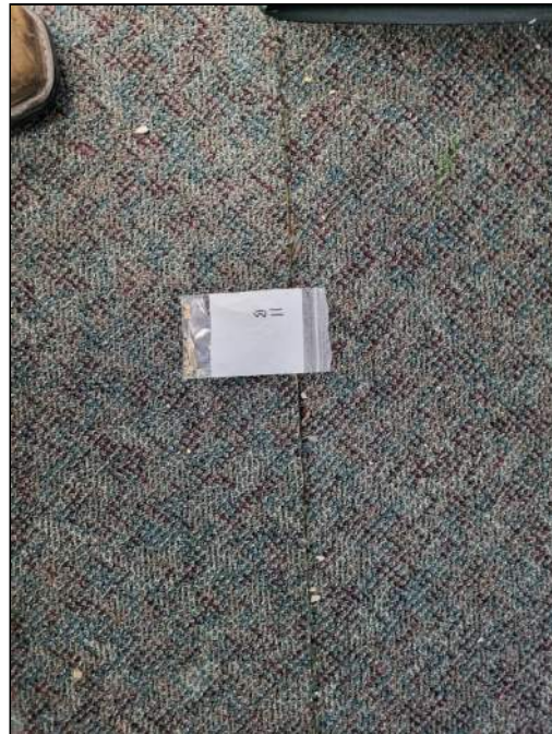
42 - Yellow Carpet Mastic with Grey Leveling Compound over Brown Mottled VFT with Black Mastic
