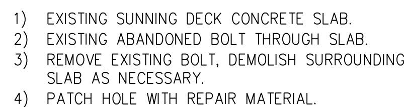
9 ABANDONED BOLT REPAIR DETAIL 1 \frac{1}{2}'' = 1'-0''
